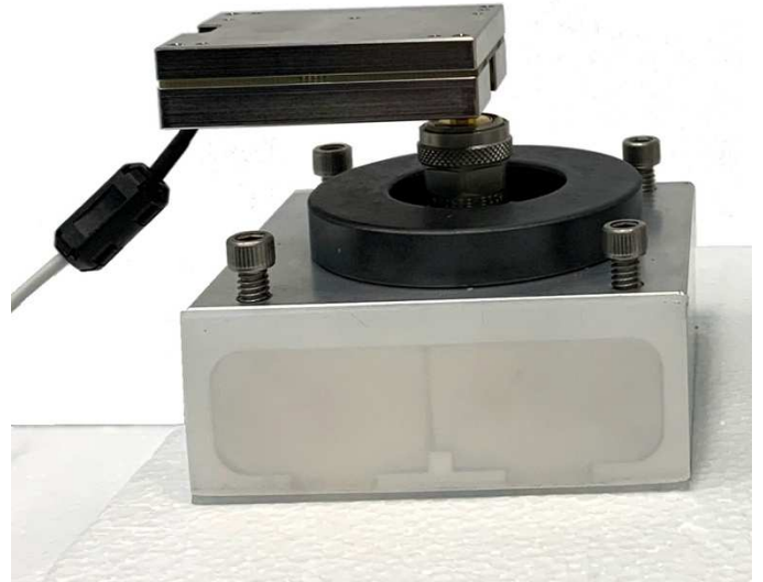
Figure 2. Photograph of open-ended stripline sensor with 1-port vector network analyzer attached.
