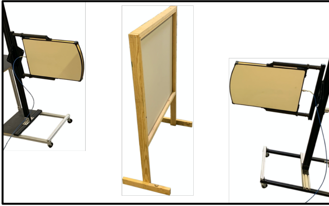
Figure 6. Photograph of two FLAT antennas on either side of a material specimen
