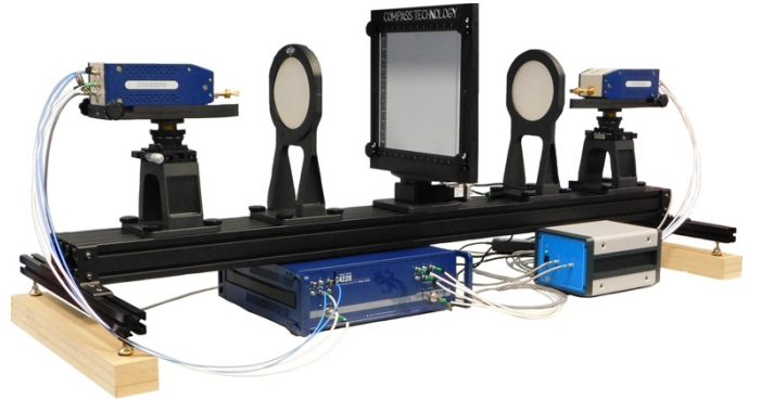
Figure 2. Photograph of lens-based focused beam system for measuring materials at 60-90 GHz.
