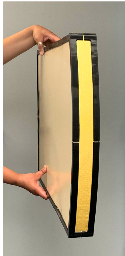
CTG's new FLAT200 antenna with horn-like directivity from 200 MHz to 4 GHz
