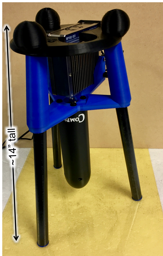
Figure 1 Photograph of an integrated 2-18 GHz reflectometer system including both sensor and a Copper Mountain Technologies RP180 vector analyzer.
