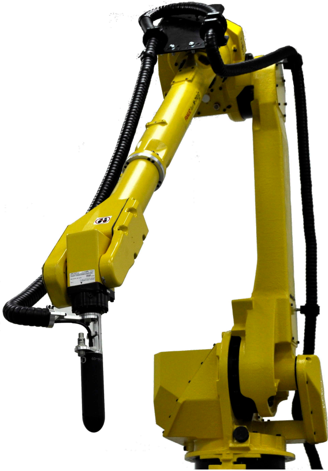
Figure 1 Photograph of robot with microwave spot probe and RF cable that must flex with robot motion.
