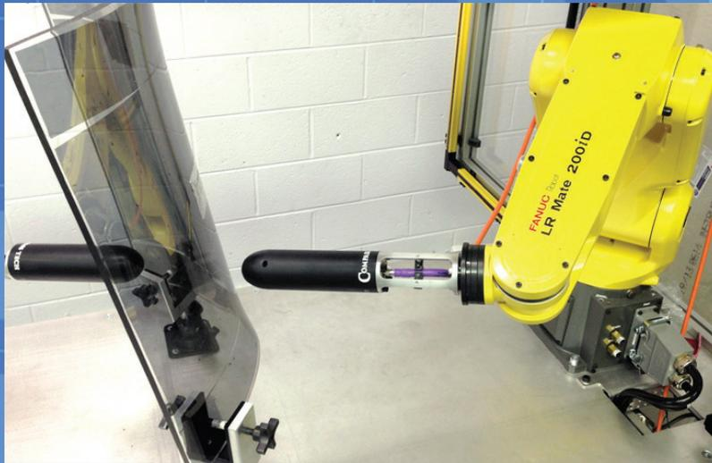
Figure 1: Microwave Mapping Transparency Sensor System (MM-TSS) Development System, showing pair of innovative broadband RF spot probes on robotic arms. (Courtesy Photo)
